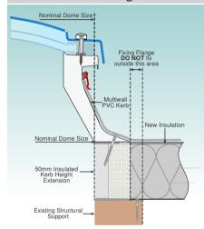
The Brett Martin Daylight Systems Kerb Heiaht Extension is a pre-coated. fully thermally broken insulated upstand that is factory supplied fitted to our propriety PVC-U kerb. The Kerb Height Extension is available in any height from 50mm-150mm and provides a simple solution to insulation suit thickness either new build or refurbishment projects.
